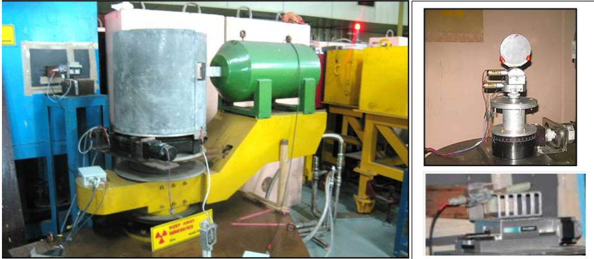
Fig. 1. Double crystal-based MSANS facility at guide tube laboratory, Dhruva. Right panel shows the micro-rotational stage and sample translation stage
