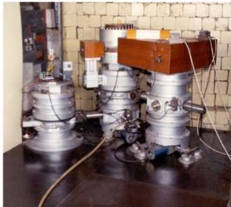
Fig. 2 Schematic and photograph of QENS spectrometer at Dhruva.
