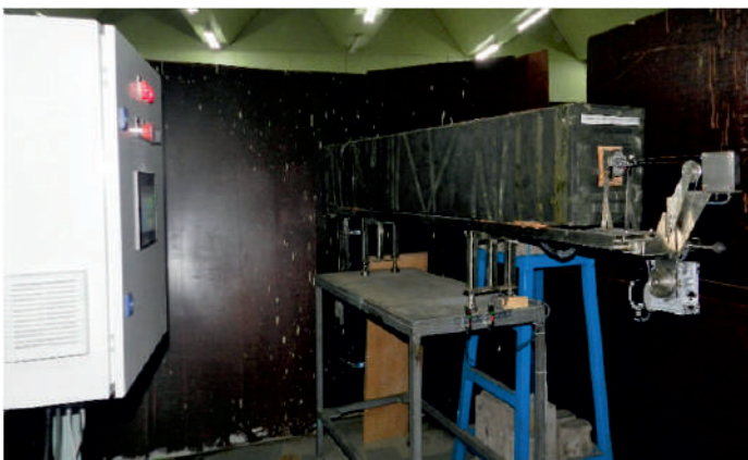
Automated X-translation at Guide G2 for precision shift of PSD
