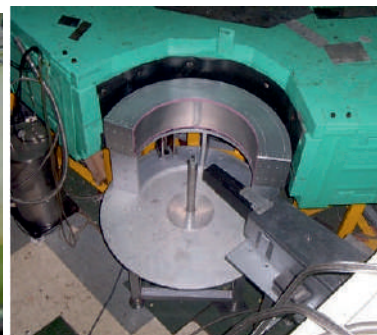
This powder diffractometer, developed and installed by UGC-DAE Consortium for Scientific Research, is a multi-PSD high throughput diffractometer.
