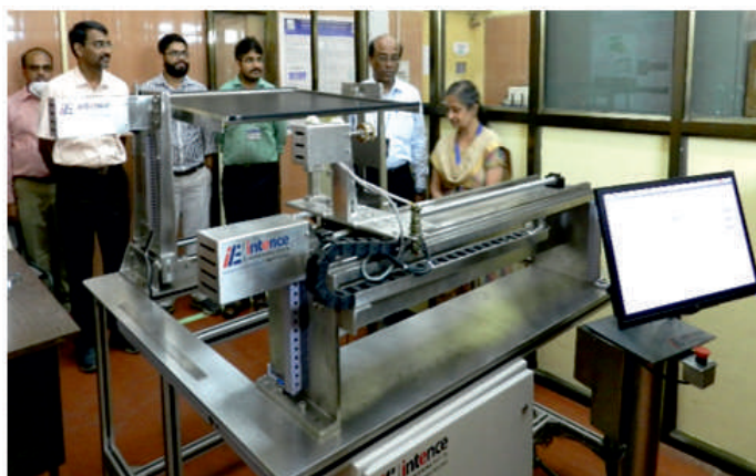
Automated Grid Winding Machine with multiwire PCB mounting frame, Linear Motion guide with control panel
