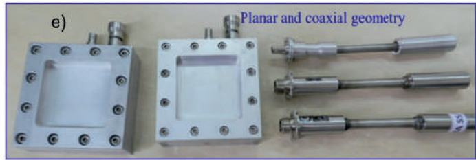
a) \text{BF}_3 filled detector for FRENA at SINP, Kolkata and RMP, Mysuru b) Neutron area monitors for Dhruva reactor c) Miniature neutron detectors for BRAHMMA neutron generator, d) Neutron detector for portable D-D neutron source e) Neutron beam monitors in planar and coaxial geometry
