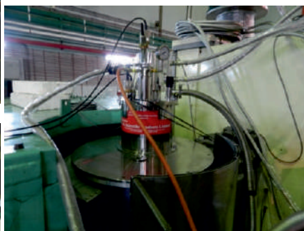
This powder diffractometer, developed and installed by UGC-DAE Consortium for Scientific Research, is a multi-PSD high throughput diffractometer.
